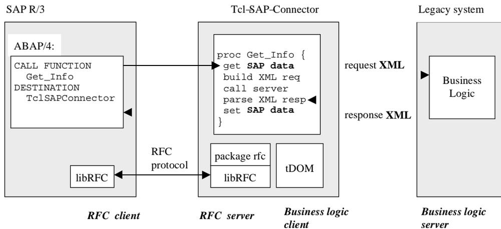
**Figure 2:** TcISAPConnector which converts RFC call in XML
